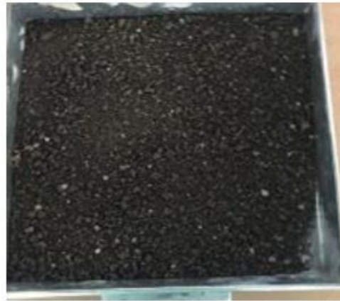
Fig 4: Steel slag as fine aggregate
