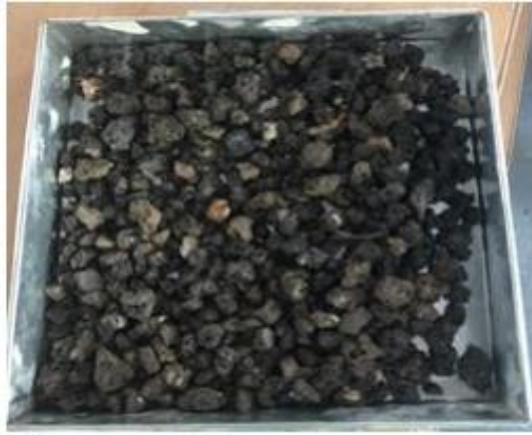
Fig 3: Steel slag as coarse aggregate
